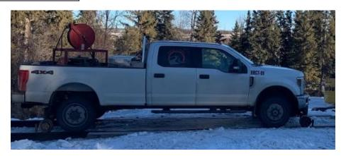
Hirail pickup trucks are the most commonly used means of travel for rail workers inspecting track. They are also used to transport crews, materials, and tools to and from worksites via rail.
