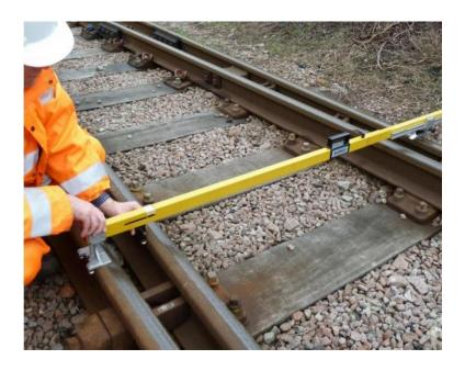
Example of a track gauge measuring tool
